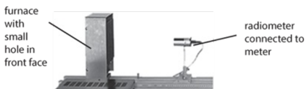
Figure 17.1: Furnace with a small hole in front face directed towards a radiometer connected to meter.
