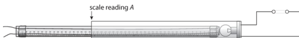
Figure 8.4: Wire on metre rule inside tube with lamp.
